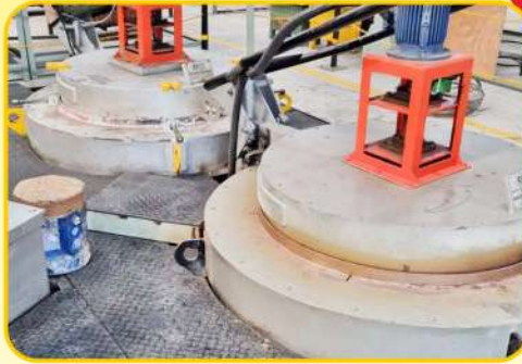
Pit Type Furnace
