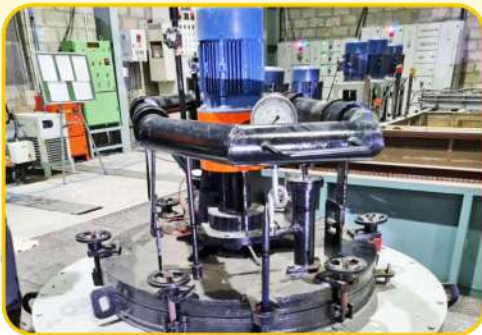
Gas Carburizing Furnace
