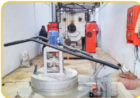
Rotary Furnace Complete Pant with Quenching Tank and Tempering Furnace
