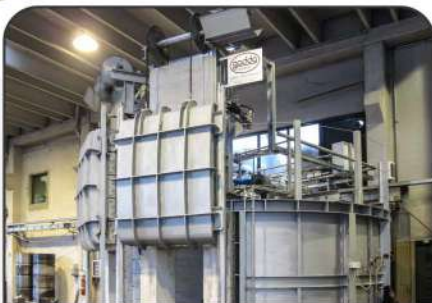
Rotary Hearth Furnace
