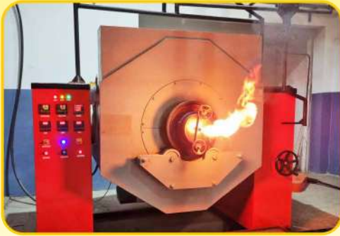
Rotary Retort Furnace
