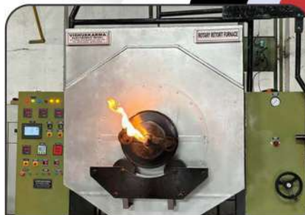
Rotary Retort Furnace
